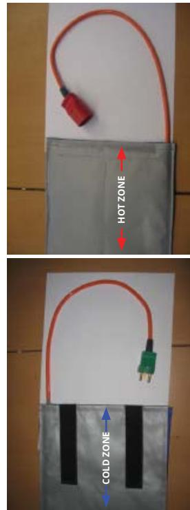
If you mount the power connector yourself always place the male connector in the cold zone of the heat blanket, and female in the hot zone
