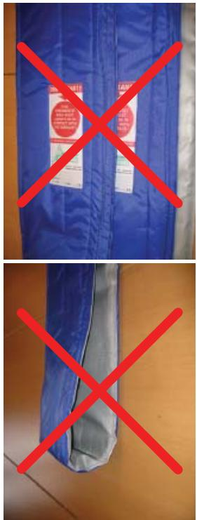
Only the area with the Velcro (cold area) must overlap. Overlap can cause fire when 2 heating areas are in contact
